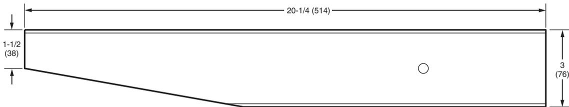
Fig. 4. S256B viewing head dimensions.
