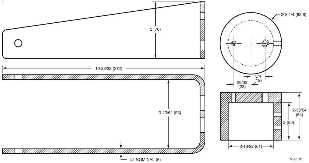
Fig. 5. Viewing head yoke and mount dimensions.
